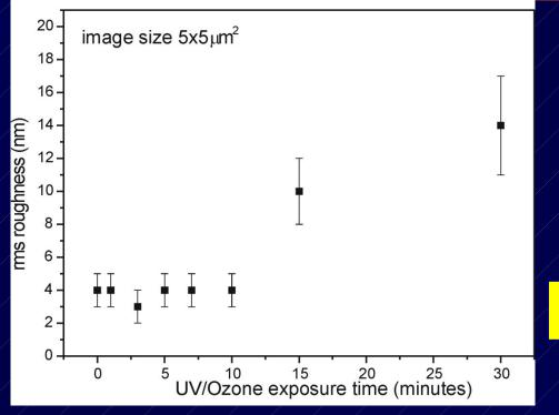
**Roughness** is constant for the first 10 minutes of UV exposure and increases after 15 minutes.
