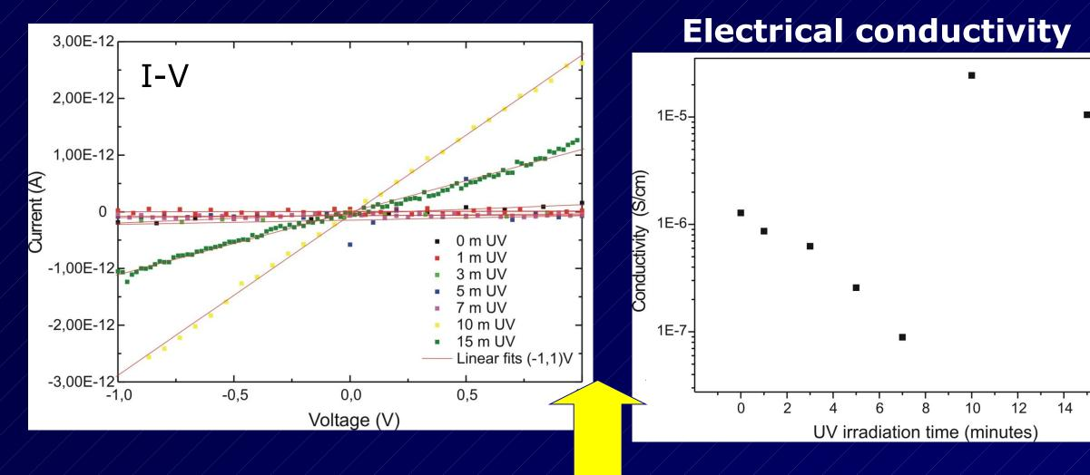
Conductivity decreases exponentially with increasing time exposure. However, after 10 minutes of exposure the conductivity increases markedly.
