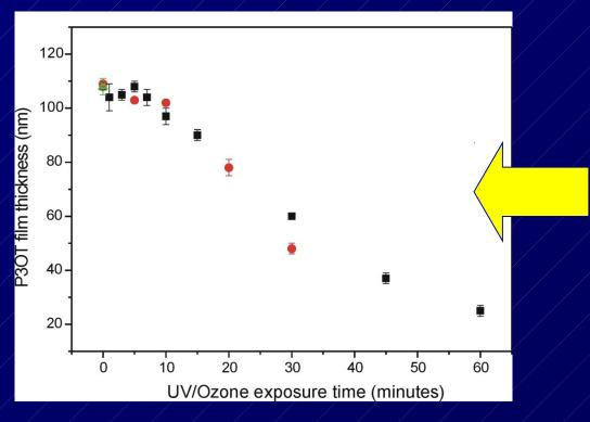
In the first **10** minutes of UV irradiation the film thickness does not change.
