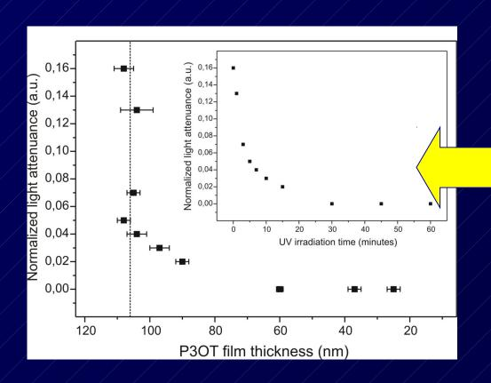
Very pronounced decrease of the light attenuace in the first minutes of exposure. However, the film thickness does not change.
