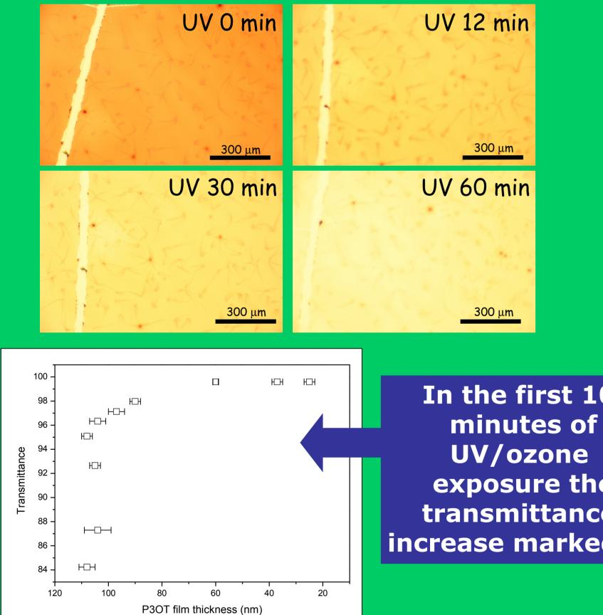
UV/ozone exposure the transmittance increase markedly After 5-7 minutes small grain like structures appear
