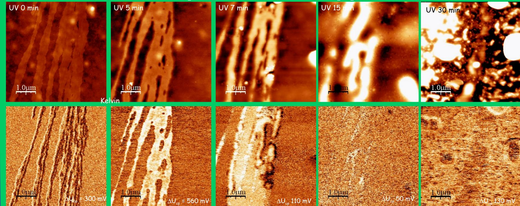
After the first UV/ozone exposure contrast of the images changes and the surface contact potential domains disappear
