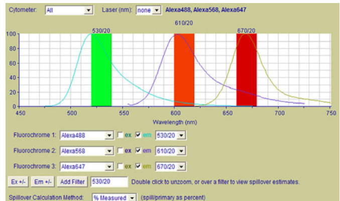
Figure 8. Screen shot of the Fluorescence Spectrum Viewer. The Fluorescence Spectrum Viewer is a useful tool for selecting appropriate probes and filter combinations for multiplexing high-content imaging applications.
