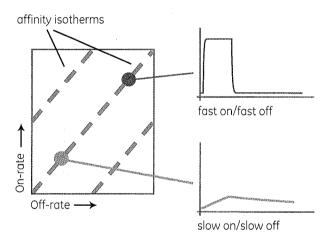
On/off-rate map showing two molecules with identical affinities, but kinetic profiles differing by several orders of magnitude. These differences could not be seen by end-point analyses.
