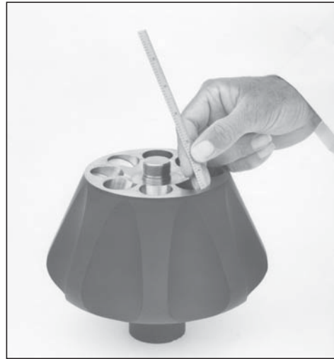
Figure 3. Measuring Distance from Cap to Rotor Tray
