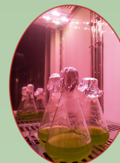
Figure 8. Experimental setup to grow Neochloris in red LED light. Growth chamber adjusted with LED light strips was used for the experiment. Growth conditions: 16:8 light:dark photoperiod, 25°C, no CO 2 addition.
