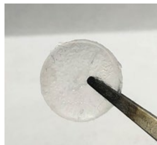
Figure 1. Ionogel formed by [Chol][TFSI] in PVDF matrix.
