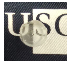
Figure 1.- Semisolid nano-encapsulated IL electrolyte in a silica scaffold.
