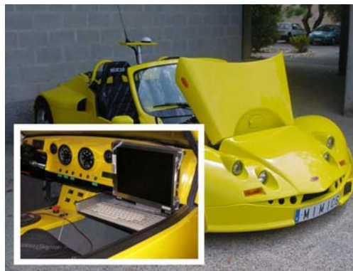
Fig. 2. Test vehicle prototype based on a roadster Comarh S1-80.
